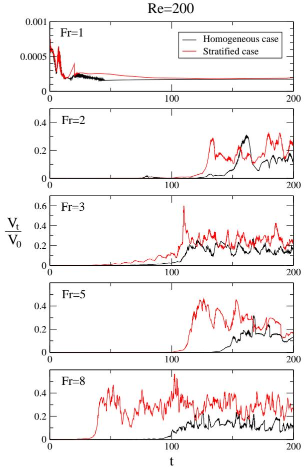
Figure 5: Time series of  $V_t/V_0$  of  $Re = 200$  fountains with varying  $Fr$  in both a homogeneous fluid and a linearly stratified fluid at  $s = 0.03$ .
