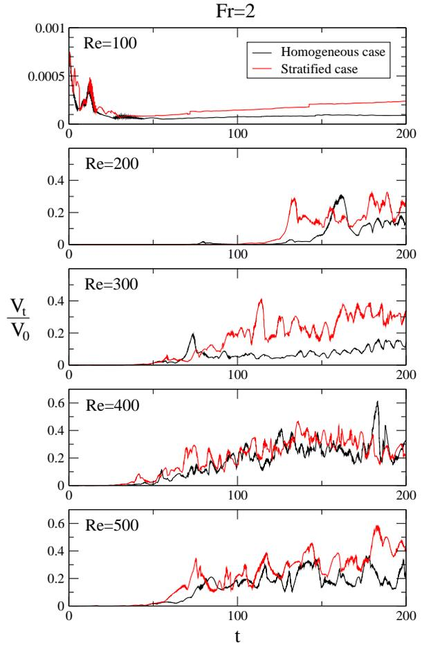
Figure 3: Time series of  $V_t/V_0$  of  $Fr = 2$  fountains with varying  $Re$  in both a homogeneous fluid and a linearly stratified fluid at  $s = 0.03$ , where  $V_t$  is the tangent velocity on the interfacial surface between the fountain fluid and the ambient fluid. The time  $t$  is made dimensionless by  $X_0/V_0$ .
