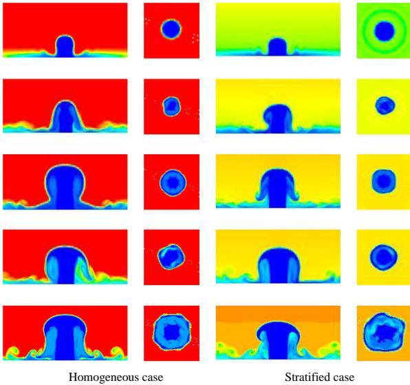
Figure 2: Steady-state temperature contours of  $Fr = 2$  fountains with varying  $Re$  in both a homogeneous fluid and a linearly stratified fluid at  $s = 0.03$ . The first and third columns are temperature contours in the vertical plane through the symmetry axis of the cylinder, and the second and the fourth columns are temperature contours in the horizontal plane at height  $Z = 0.5Z_{m,i}$ . The top to the bottom rows correspond to  $Re = 100, 200, 300, 400$  and  $500$ , respectively.
